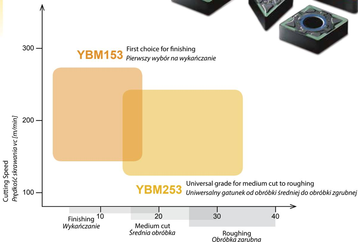
**Solution for stainless steel and materials which are hard to machine**
